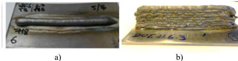
Figure 2. a) single layer b) multi layer deposition
