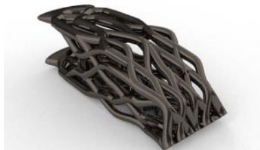
Figure 1. Generative Topology Optimization of typical 3D beam geometry
