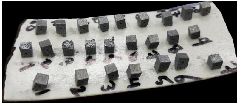
Fig 1. Additively manufactured 22 samples of AlSi10Mg.
