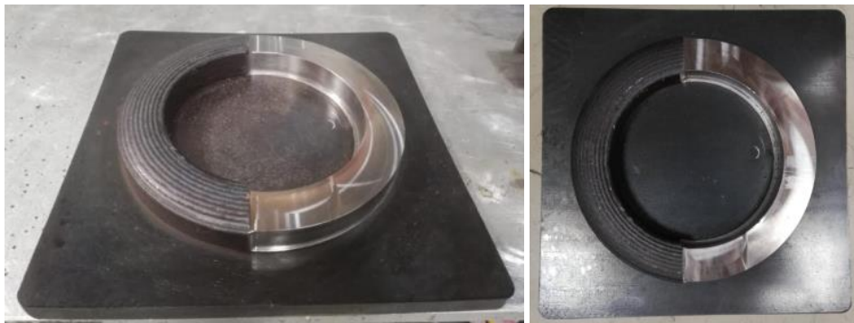
Figure 2. Produced ring geometry with WAAM
