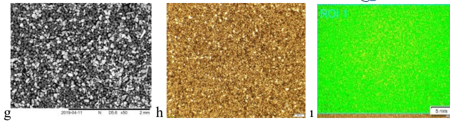
Figure 2. SEM images after mixing (50x) a. Ta-60Ti d. Ta-50Ti g. Ta-40Ti, Optic microscope images after raking by UPB (5x) b. Ta-60Ti e. Ta-50Ti h. Ta-40Ti, OLYMPUS Stream software report c. Ta-60Ti f. Ta-50Ti i. Ta-40Ti.
